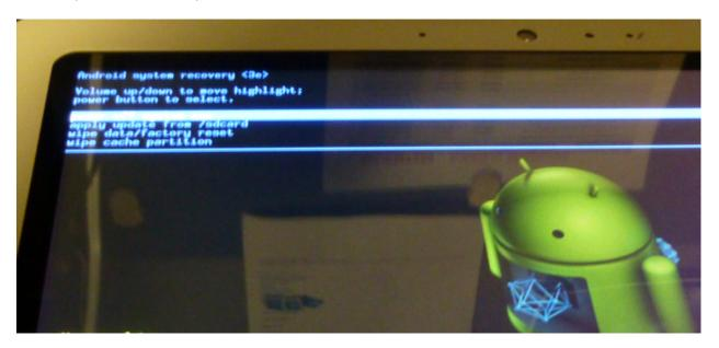
In recovery mode, the Home button(center screen bottom) is used to Enter and Volume up and down keys are used to select the line.
