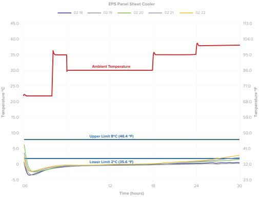
5. The EPS Molded Cooler held temperature for 18 hours; thermal excursions occurred during the 18 to 24 hour interval during summer profile testing.
