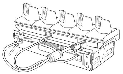
11. Secure top tray to bottom tray with 4 M5 screws (two on each side).
