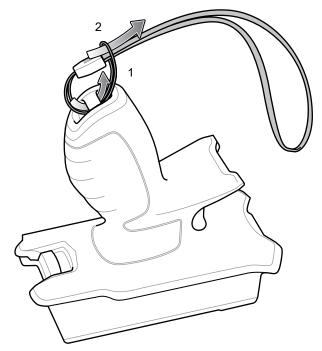
3. Pull the lanyard until the loop tightens.
