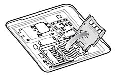
**4.** Insert the microSD card into the card holder door ensuring that the card slides into the holding tabs on each side of the door.
