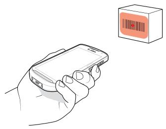
Press and hold the scan button.The red laser aiming pattern turns on to assist in aiming.
