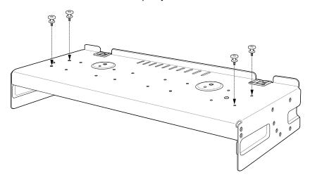
7. Align and install 5-Slot cradle onto studs of top tray.
