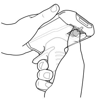
2. Slide the device forward and then rotate the bottom of the device up.
