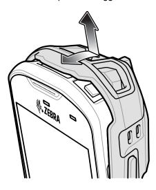
3. Push the device into the Rugged Boot.
