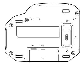
For Ethernet communication, slide the switch to the \*\* position.
