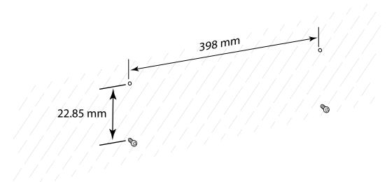
3. Align the mounting bracket's bottom mounting key holes with the screws.
