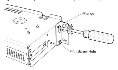
Figure 70 Flange 25° Position (4-Slot Battery Chargers)
