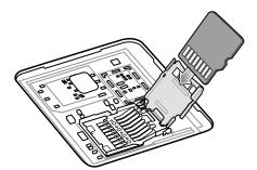
5. Close the microSD card holder and slide into the lock position.
