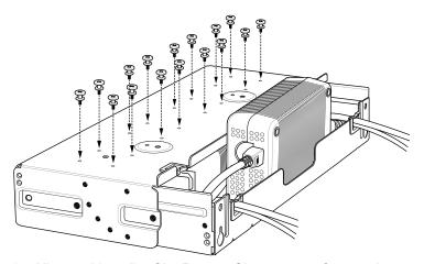
9. Align and install 4-Slot Battery Charger onto four studs.
