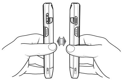
When the devices connect, a sound emits, the image on the screen reduces in size, the message **Touch to beam** displays.
