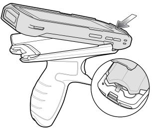
2. Rotate the device down and press down until it snaps into place.
