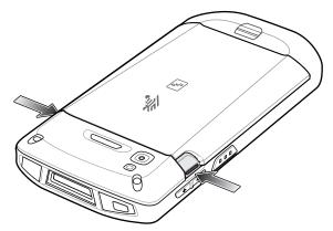
7. Lift the battery from the device.
