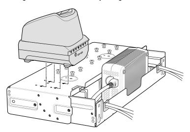
**10.**Connect DC Y cables to four 4-Slot Battery Chargers.
