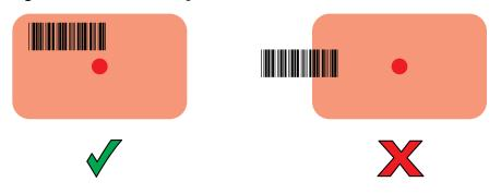
Figure 29 DS3678 Pick List Mode with Multiple Barcodes in Aiming Pattern
