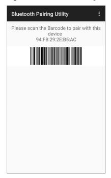
2. Using the Ring Scanner, scan the barcode on the screen.
