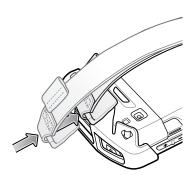
7. Push the clip onto the top cap.
