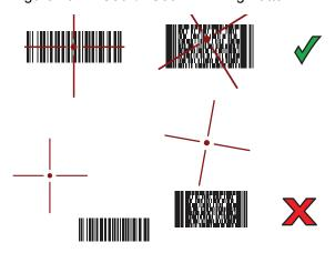
Figure 20 RS507/RS507X Pick List Mode with Multiple Barcodes in Aiming Pattern
