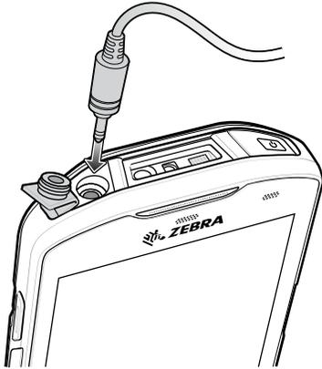
3. Insert the 2.5 mm headset plug into the jack on the Audio Adapter.
