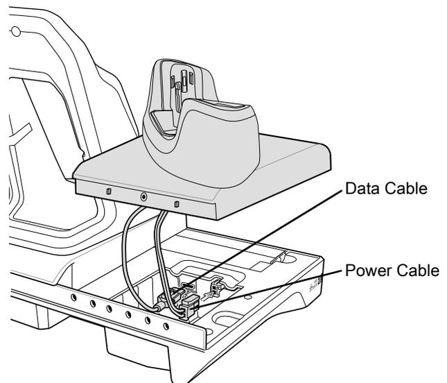
6. Place the data cable in the cable channel and under the cable retention tab on the cradle base.
