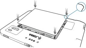
Carefully press down around the edges of the cover. Make sure that the cover is seated properly.
