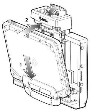
**4.** Use your thumb to push the tablet into the dock, then push the lever down to secure the tablet.
