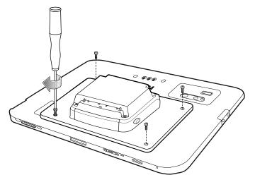
**NOTE:** The engraved arrow on the expansion back indicates the location of the card contacts.
