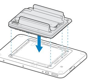
Using a cross head or Phillips screwdriver, secure the payment Z back to the device using three M2 11 mm and two M2 4 mm screws.
