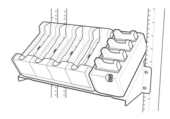
8. Slide the the cradle and the charger down onto the tabs.
