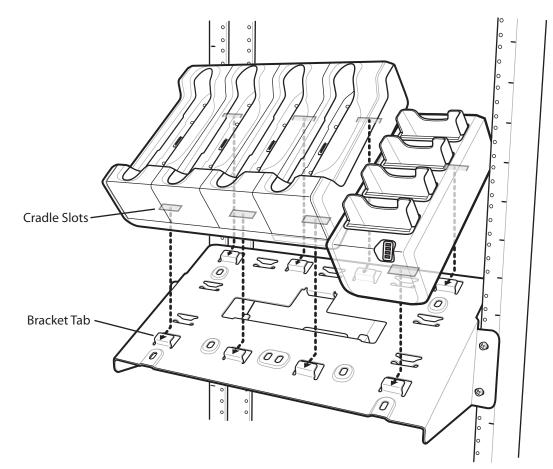
7. Align the slots on the bottom of the Four-slot Charge Only Cradle and the Four-slot Battery Charger with the tabs on the bracket.
