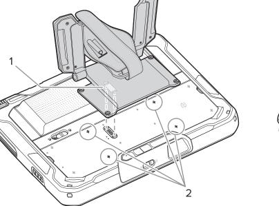
Secure the Kick-Stand to the tablet using four screws. Torque to 4.5 kgf-cm (3.9 lbf-in.).
