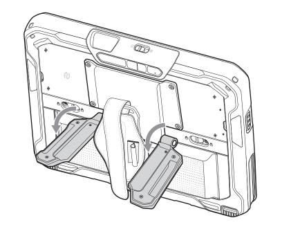
Place the tablet on a flat surface and adjust viewing angle.
