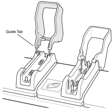
2. Place the guide down onto the cradle and then rotate the guide until it snaps into the cradle.
