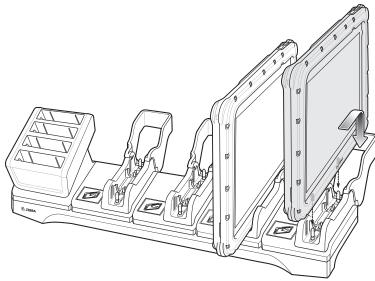
Place the ET5X down into the slot with display facing away from Battery Charger.
