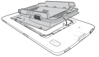
Rotate the Payment Sled down into the battery well.
