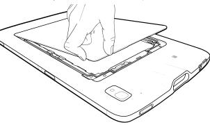
Insert the tabbed end of the Payment Sled into the battery well. Ensure that the tabs on the Payment Sled are aligned with the slots in the battery well.
