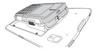
Lift the top clip and tighten the security screw. Torque to 14 n-cm.
