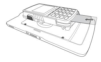
Place your hand between the device and the hand strap and adjust the hand strap as necessary.
