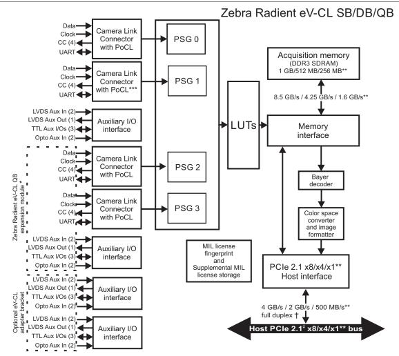
\* Note that, without the expansion module, this is a flow diagram of Zebra Radient eV-CL SB or DB, depending on the number of camera link interfaces. With the expansion module, this is a flow diagram of Zebra Radient eV-CL QB. eV-CL SB and DB are not upgradable to eV-CL QB; the eV-CL SB and DB do not have the required connector for the eV-CL QB module.
