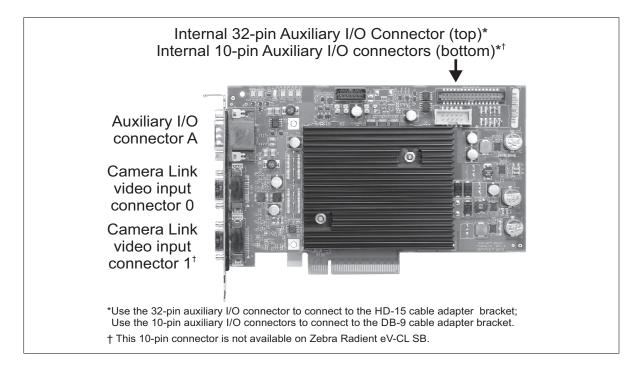
On the Zebra Radient eV-CL cable adapter bracket, there is either two HD-15 auxiliary I/O connectors or one DB-9 auxiliary I/O connector<sup>\*</sup>; these allow you to access the signals of the internal auxiliary I/O connector from outside the computer enclosure. See the *External auxiliary I/O connectors* section below for information on how to connect these adapter brackets.
