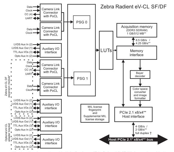
\* Note that, without the expansion module, this is a flow diagram of Zebra Radient eV-CL SF. With the expansion module, this is a flow diagram of Zebra Radient eV-CL DF. eV-CL SF is not upgradable to eV-CL DF; the eV-CL SF does not have the required connector for the eV-CL DF module.
