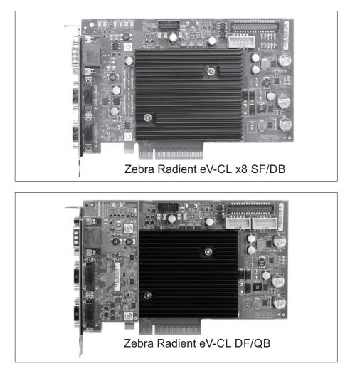
Note that older versions of Zebra Radient eV-CL included a fan. This has been replaced with a heat sink in newer versions.
