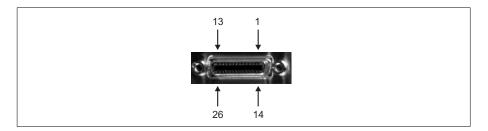
The number of Camera Link video input connectors and their pinout depends on the version of Zebra Radient eV-CL and the configuration. The pinout of these connectors follows the Camera Link standard.
