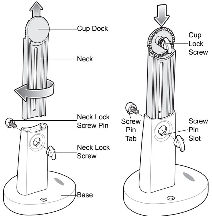
1. Turn the neck lock screw counterclockwise and remove the neck lock screw and neck lock screw pin.
