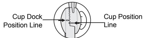
**IMPORTANT:** For proper document capture, the position lines on the cup and the cup dock should appear as shown in the diagram above. The position line on the cup dock should be one groove above the position line on the cup.
