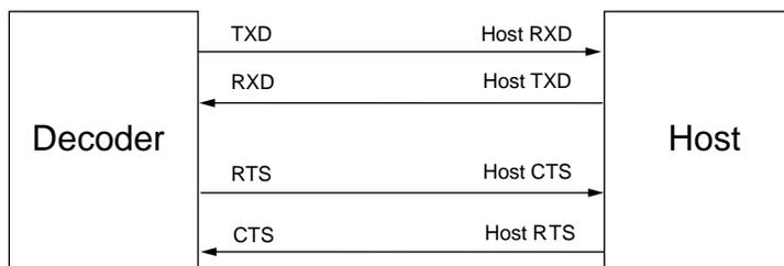
**Figure 1-1** Host/Decoder Interconnection
