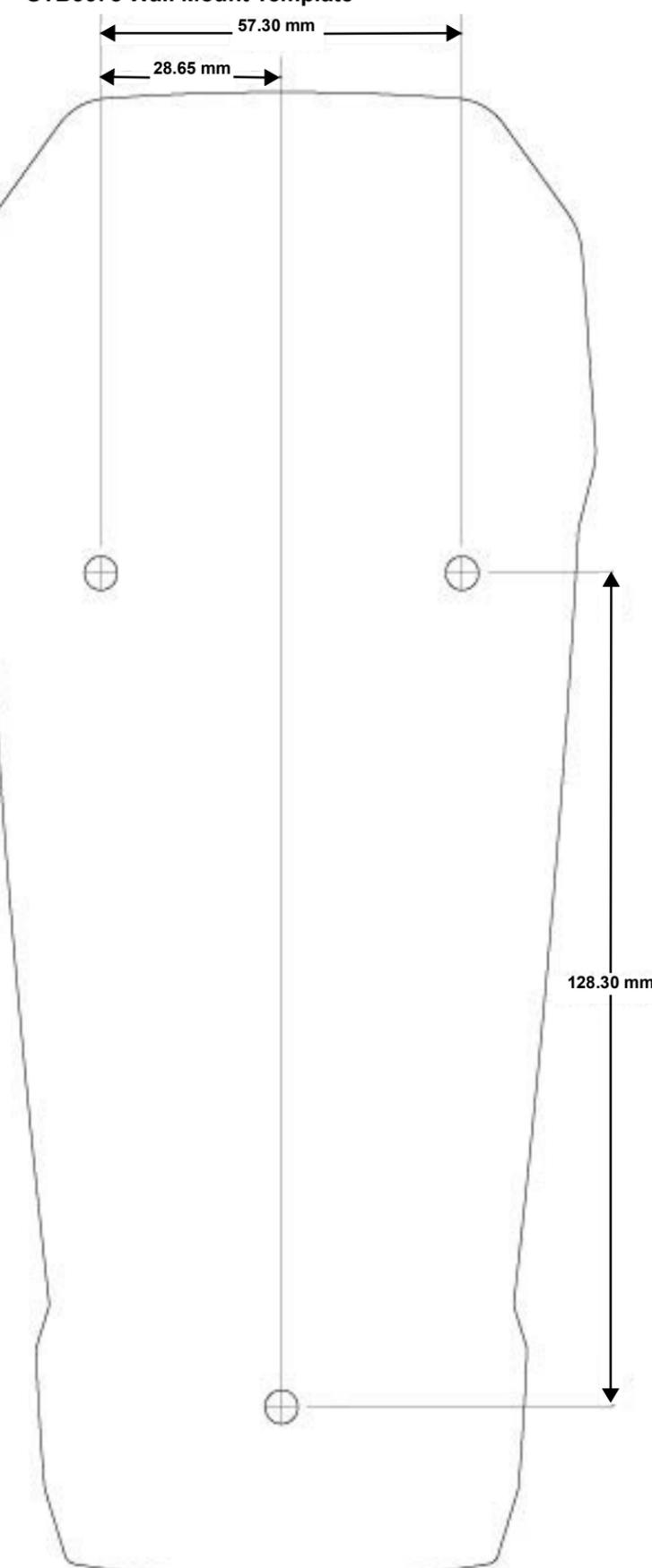
**NOTE** When printing the STB3678 QRG which includes the wall mount template, ensure the dimensions print correctly by setting the **Page Sizing and Handling to Actual Size**.
