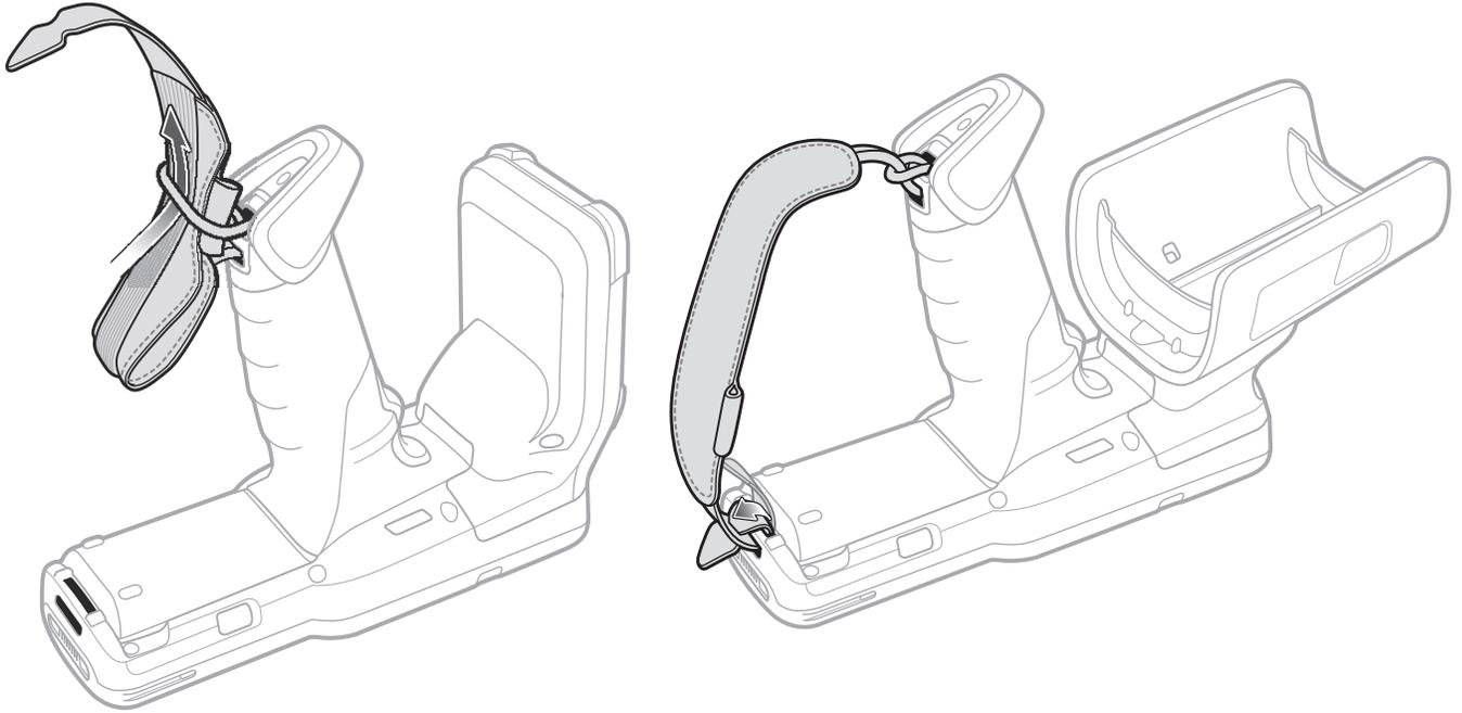
6. Slide the tab through the slit in the hand strap so that the tip of the tab is facing away from the MC3300xR.
