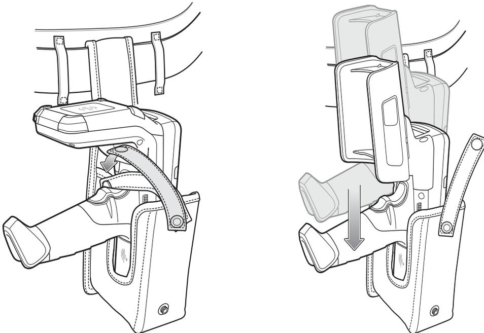
3. Secure the MC3300xR with the restraining strap and place over the MC3300xR to secure in place.
