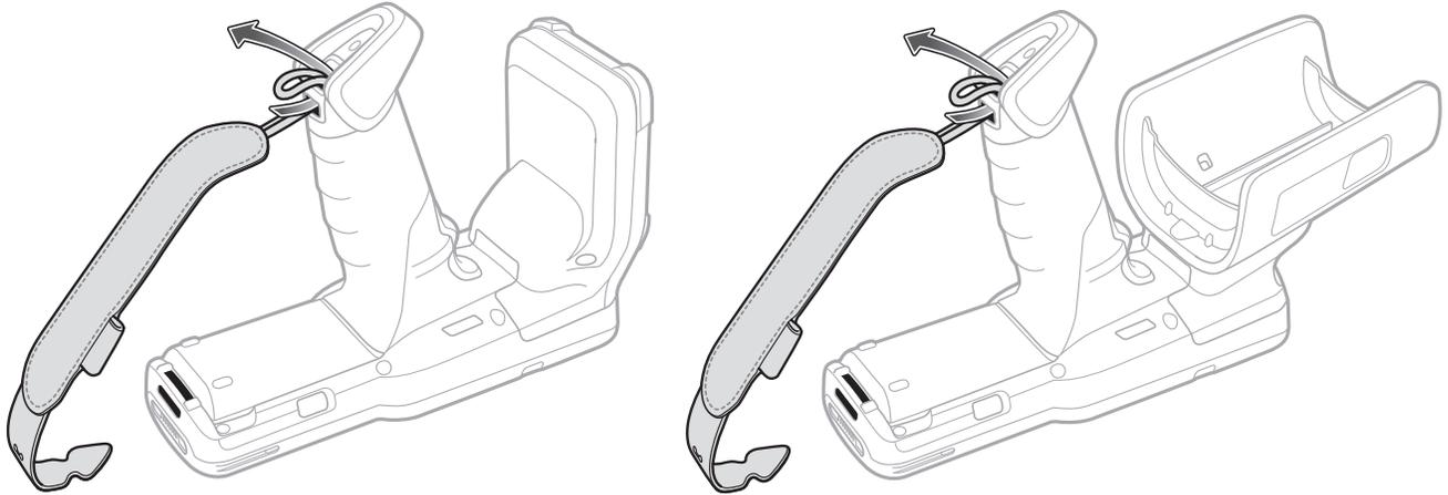
2. Insert the top end of the hand strap through the loop.
