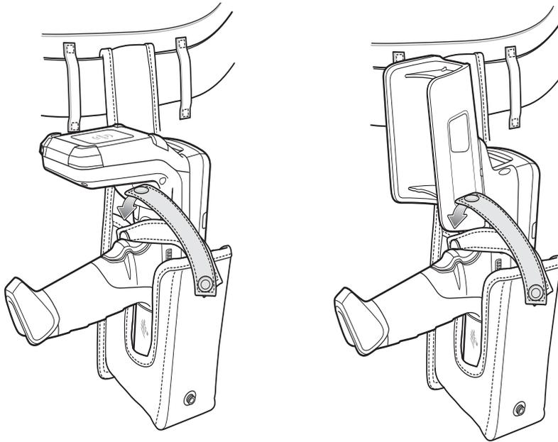
4. To remove the MC3300xR, unsnap the restraining strap to release. Lift the MC3300xR out of Fabric Holster.
