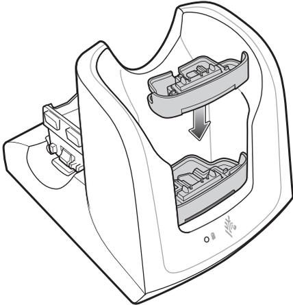
4. Insert the MC3300xR device into the MC32N0 cradle.
