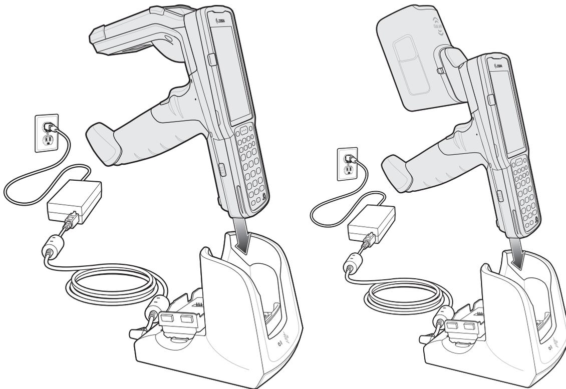
The MC3300xR 5200 mAh and 7000mAh PowerPrecision+ extended battery charges from 0% to 90% in less than 5.5 hours at room temperature.
