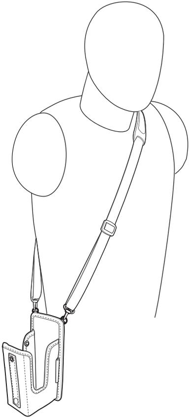
3. Lift the strap and insert the MC3300xR into the holster.
