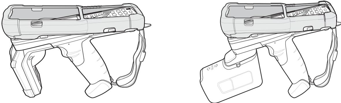
3. Grasp the top of the rubber boot and place over the top of the MC3300xR.
