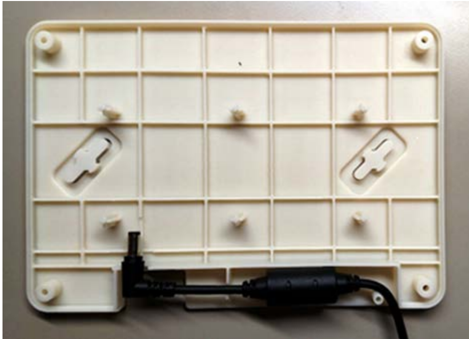
Figure 37 Routing Power Cable
