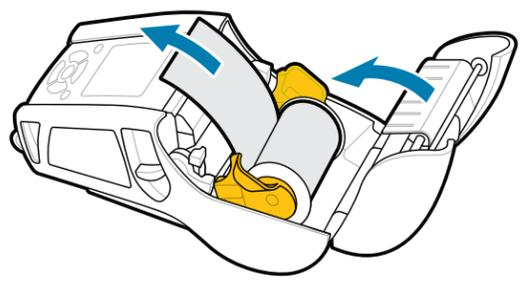
3. Close the media cover making sure to manually feed the end of the media roll outside the printer.
