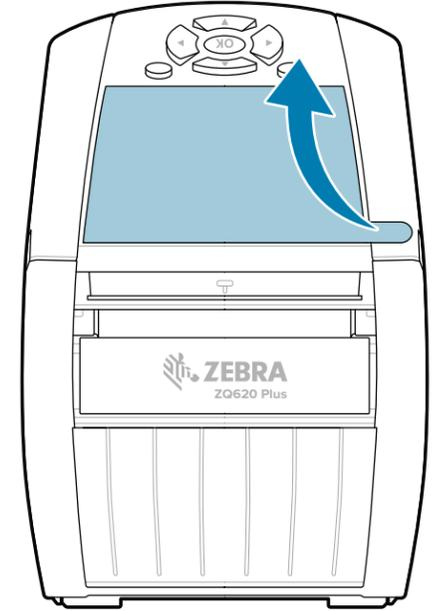
④ Removing the Battery
