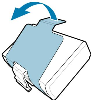
4. Peel back the tape insulator and remove it from the top of the battery pack. Discard upon removal.
