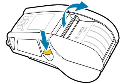
1. Press down on the latch release to open the media cover.
