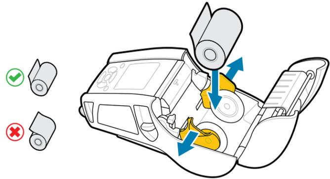
2. Insert the media roll in the media compartment in the orientation shown.
