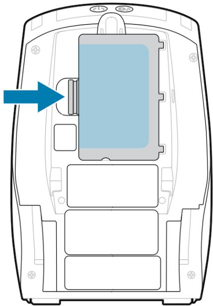
1. Press the release tab on the battery pack.
