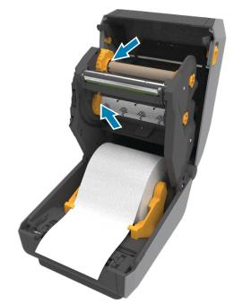
Place the left side of the spool onto the spindle aligning it with the notches.
