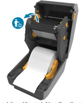
Open the printer and discard the used ribbon. Keep the empty supply spool to use for the next the ribbon take-up.
