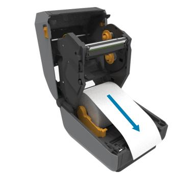
Pull the end of the roll past the front edge of the printer.
