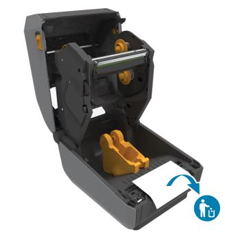
Open the printer and remove the packing.
