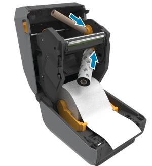
Push the right side of the spool onto the spring-loaded spindle.
