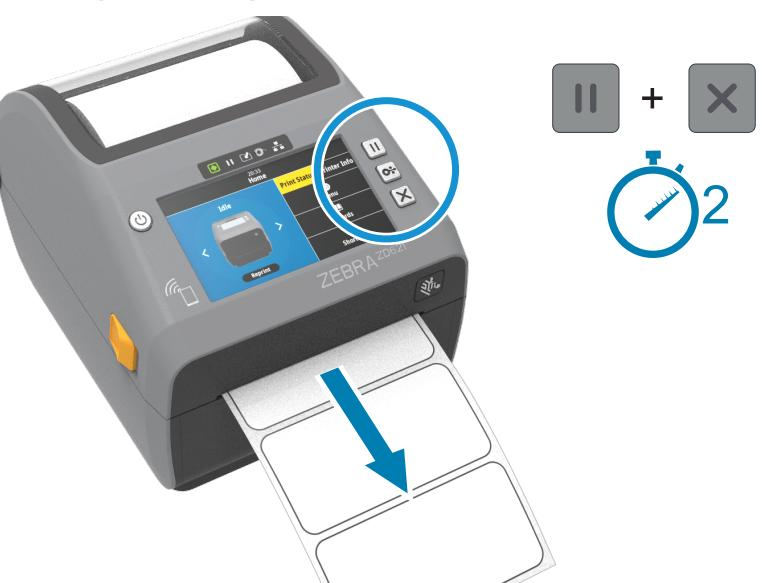
Press and hold the Pause and Cancel buttons for two seconds to line up the labels.
