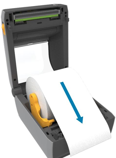
Pull the end of the roll past the front edge of the printer.
