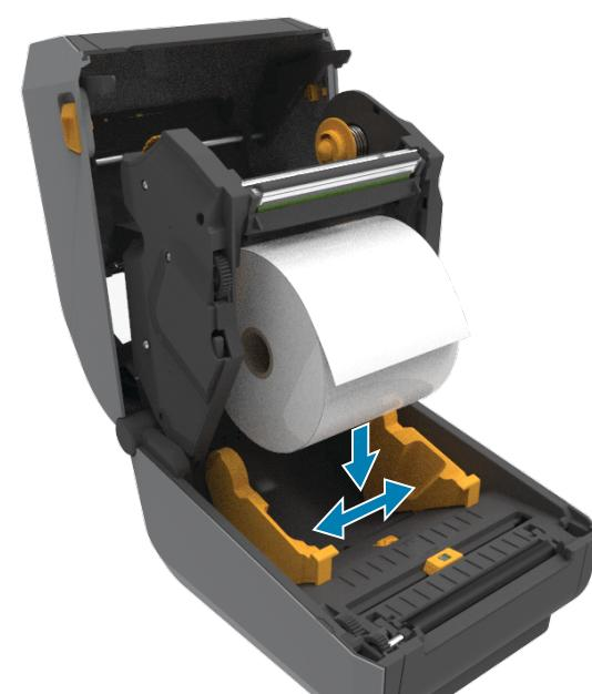
Spread the roll holders open and place the roll into the printer.
