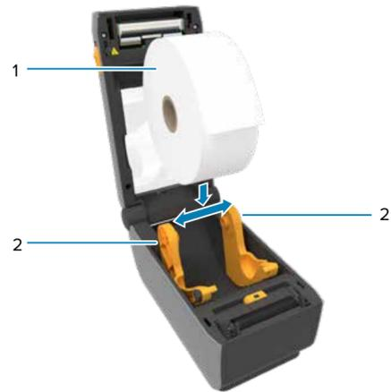
Spread the roll holders (2) open and place the roll (1) into the printer.
