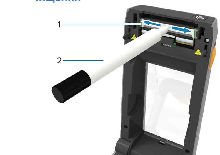
Clean printhead (1) with a cleaning pen (2). Clean from the middle to the outside. The cleaning pen is only for cleaning a printhead.
