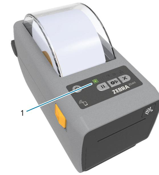
When the the printer is ready, the printer status light (1) will turn green.
