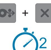
Press and hold the Feed (1) and Cancel (2) buttons for two seconds to print a configuration report.
