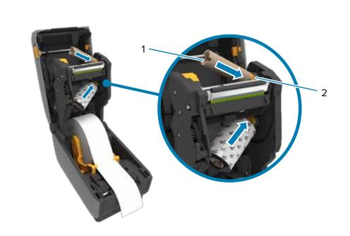
Push the right side of the spool (1) onto the spring-loaded spindle (2).
