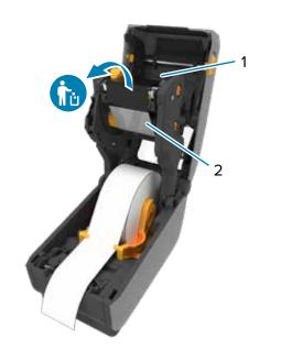
Open the printer and discard the used ribbon. Keep the empty supply spool (2) to use for the next the ribbon take-up (1).
