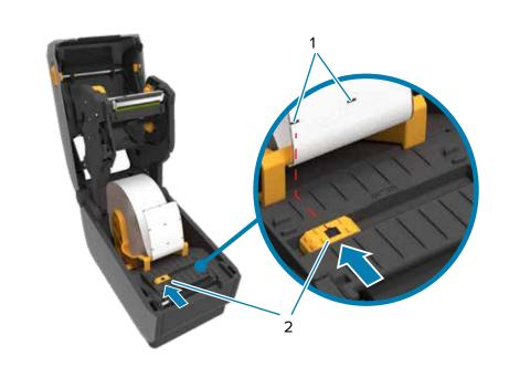
Align the sensor (2) to marks (1) away from the center of the roll for marked labels.
