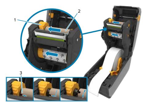
Place the left side of the spool (2) on the spindle (1) aligning it with the notches (3).
