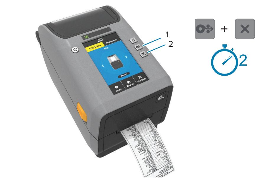
Press and hold the Feed (1) and Cancel (2) buttons for two seconds to print up the labels.
