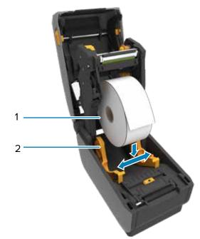
Spread the roll holders (1) open and place the roll (2) into the printer.
