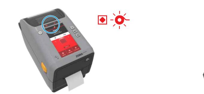
When the ribbon runs out, the printer status and a flashing media status lights (1) will turn red.
