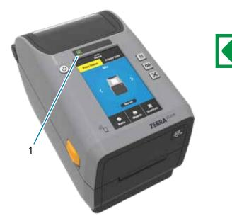
When the the printer is ready, the printer status light (1) will turn green.
