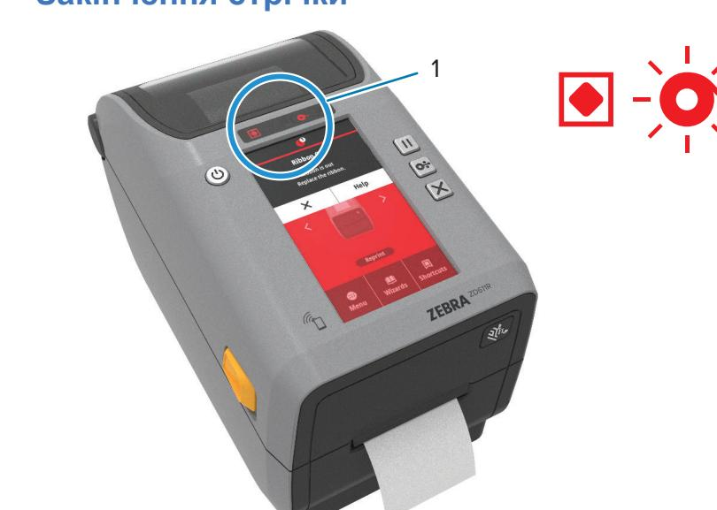
When the ribbon runs out, the printer status and a flashing media status lights (1) will turn red.
