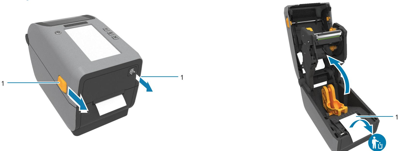
Slide the release latches (1) to the front to unlock the cover.
