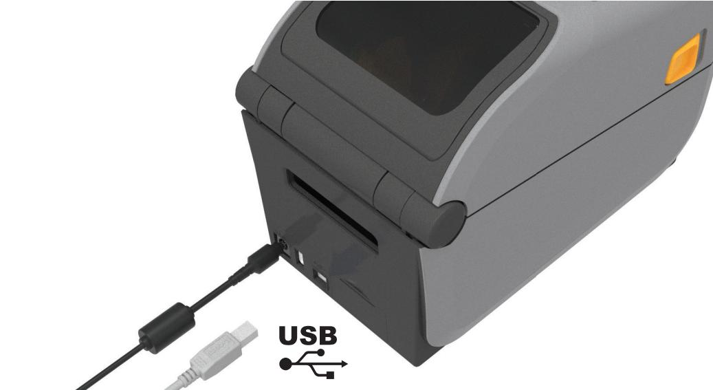
Connect a USB cable to the printer, connect the other end to your computer.
