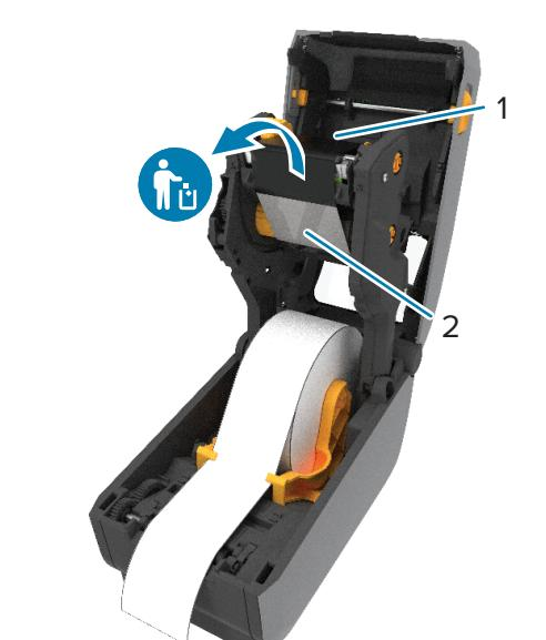
Open the printer and discard the used ribbon. Keep the empty supply spool (2) to use for the next ribbon take-up (1).
