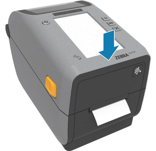
Press down on the front edge of the printer until it locks.
