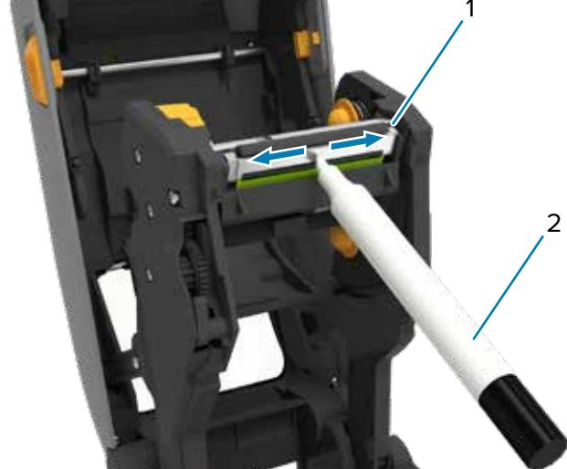
Clean printhead (1) with a cleaning pen (2). Clean from the middle to the outside. The cleaning pen is only for cleaning a printhead.
