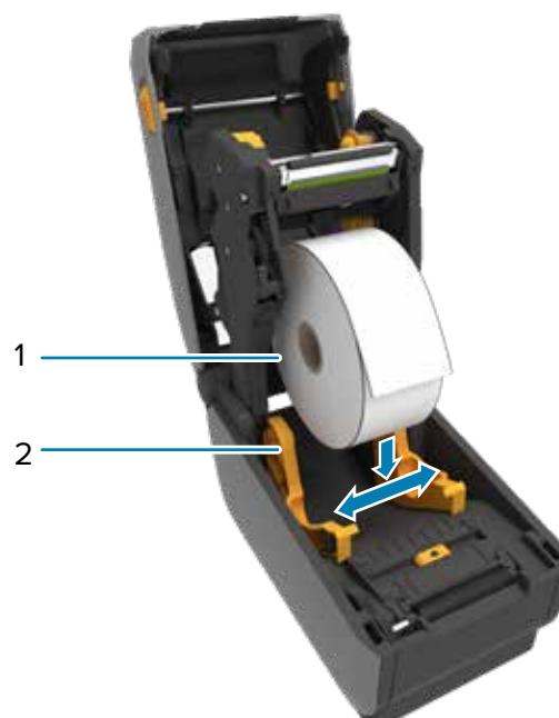
Spread the roll holders (1) open and place the roll (2) into the printer.
