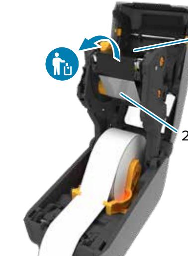
Open the printer and discard the used ribbon. Keep the empty supply spool (2) to use for the next ribbon take-up (1).
