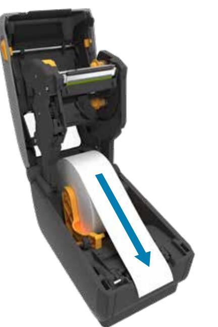
Pull the end of the roll past the front edge of the printer.
