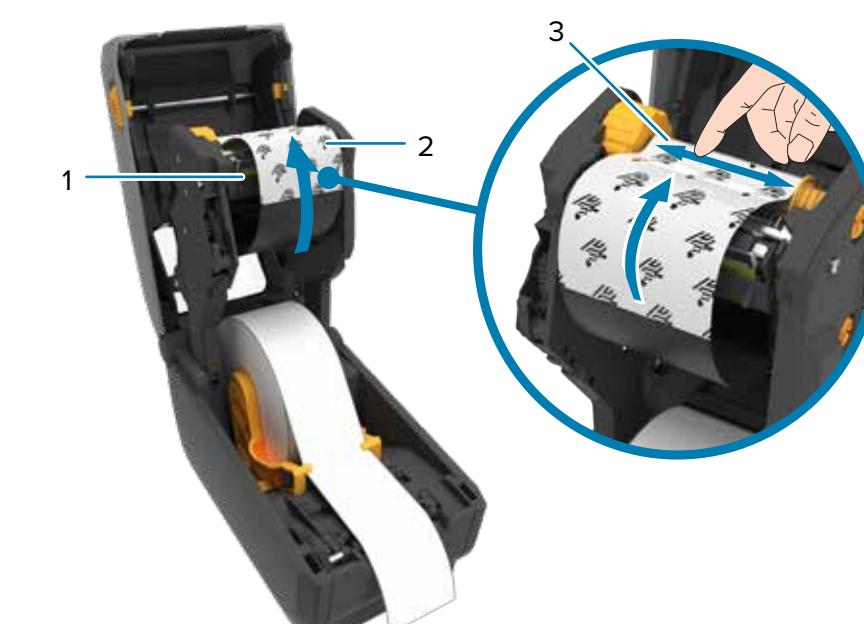
Pull the supply ribbon leader (2) up and over the printhead (1) and attach it to the take-up spool (3).
