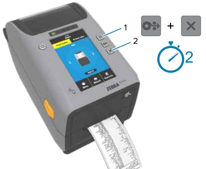
Press and hold the Feed (1) and Cancel (2) buttons for two seconds to print a configuration report.
