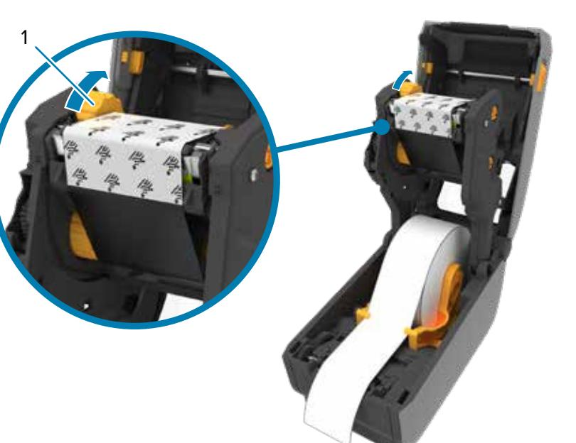
Turn the ribbon take-up wheel (1) to remove the slack and advance the ribbon.
