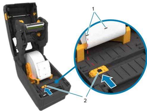
Align the sensor (2) to marks (1) away from the center of the roll for marked labels.
