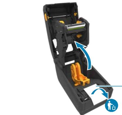
Open the printer and remove the packing (1).
