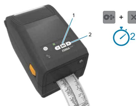
Press and hold the Feed (1) and Cancel (2) buttons for two seconds to print a configuration report.
