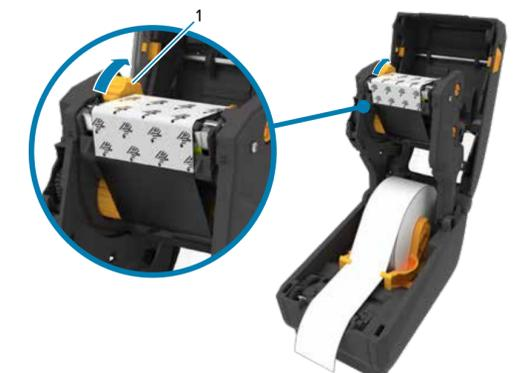
Turn the ribbon take-up wheel (1) to remove the slack and advance the ribbon.
