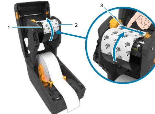
Pull the supply ribbon leader (2) up and over the printhead (1) and attach it to the take-up spool (3).
