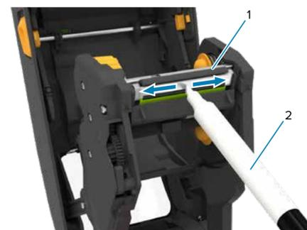
Clean printhead (1) with a cleaning pen (2). Clean from the middle to the outside. The cleaning pen is only for cleaning a printhead.
