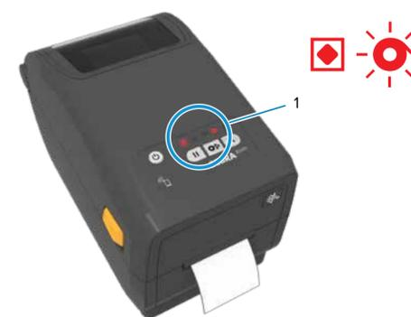
When the ribbon runs out, the printer status and a flashing media status lights (1) will turn red.
