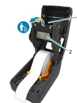
Open the printer and discard the used ribbon. Keep the empty supply spool (2) to use for the next the ribbon take-up (1).
