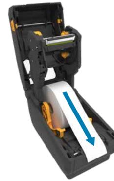
Pull the end of the roll past the front edge of the printer.
