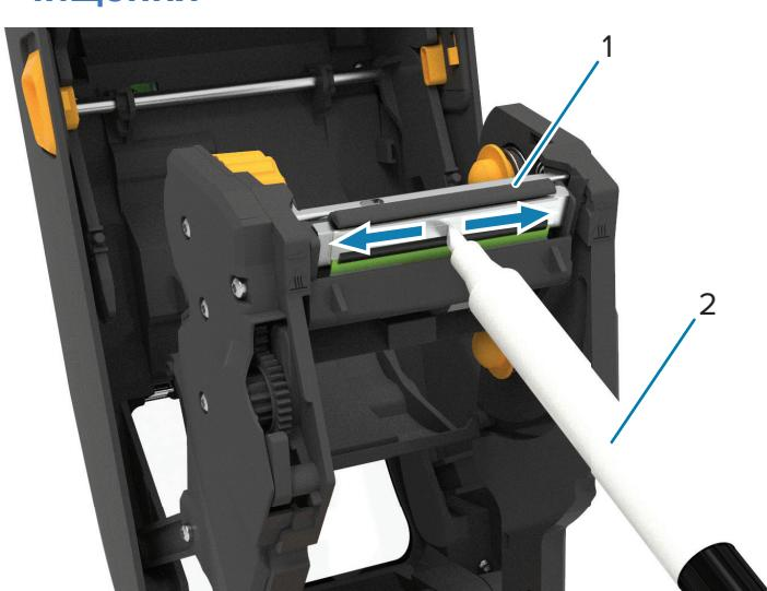
Clean printhead (1) with a cleaning pen (2). Clean from the middle to the outside. The cleaning pen is only for cleaning a printhead.
