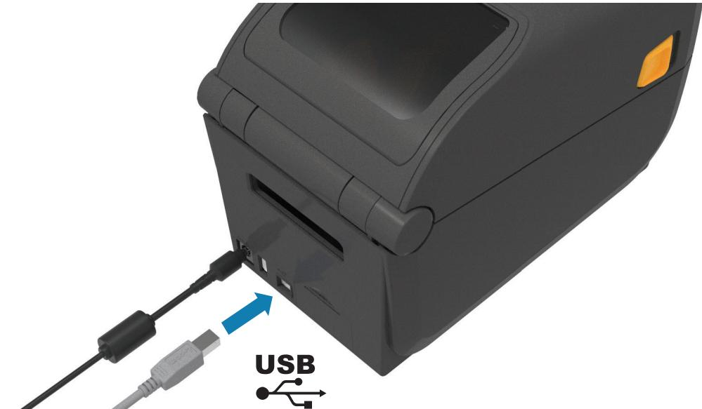
Connect a USB cable to the printer, connect the other end to your computer.
