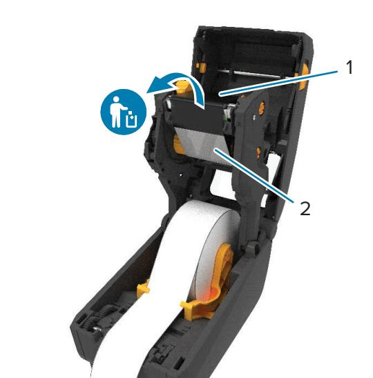
Open the printer and discard the used ribbon. Keep the empty supply spool (2) to use for the next ribbon take-up (1).
