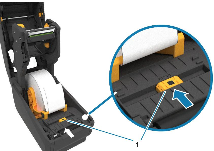
Spread the roll holders (1) open and place the roll (2) into the printer.
