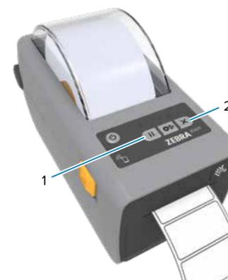
Press and hold the Pause (1) and Cancel (2) buttons for two seconds to line up the labels.
