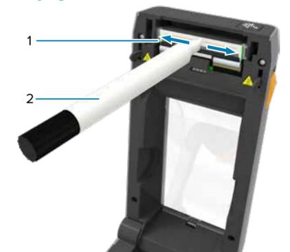
Clean printhead with a cleaning pen. Clean from the middle to the outside. Do not use a cleaning pen on the platen.
