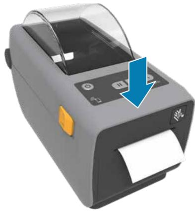
Press down on the front edge of the printer until it locks.
