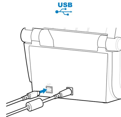
Connect the USB cable to the printer.
