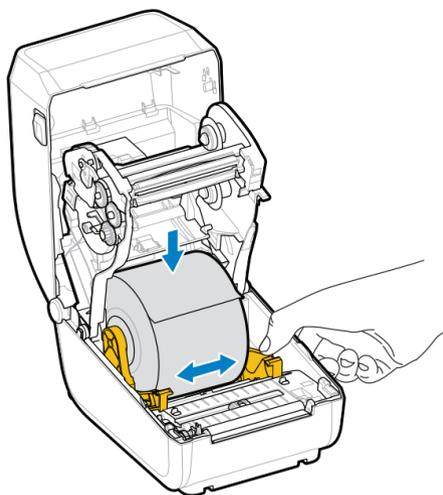
Pull the media guides open and place the media roll on the roll holders.
