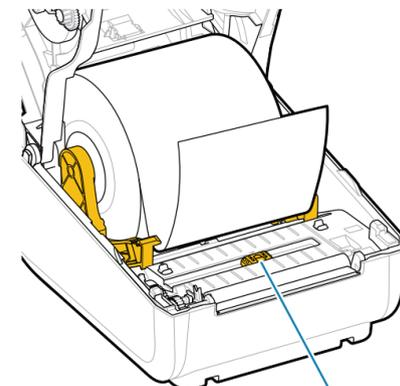
Align the sensor (1) near the center (default).
