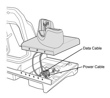
6. Place the data cable in the cable channel and under the cable retention tab on the cradle base.
