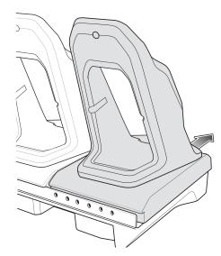
4. Disconnect the Ethernet cup cables (power and data) from the connectors.
