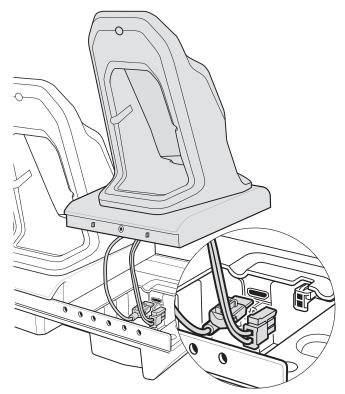
5. Connect the replacement TC5/TC7 cup cables (power and data) to the cradle connectors.
